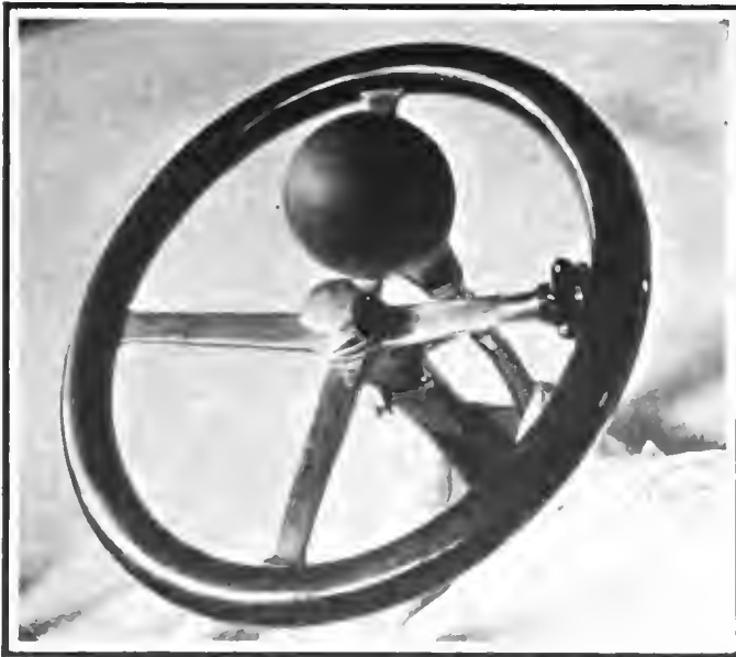
Lancia Steering Wheel showing a rotary star shaped member concentric with one of the arms adjacent to the rim by means of which the mixture is adjusted to suit the requirements—ignition is fixed and requires no controlling lever
